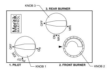
NOTE: Knob cannot be turned from "PILOT" to "OFF" unless knob is pushed in slightly. Do not force.
